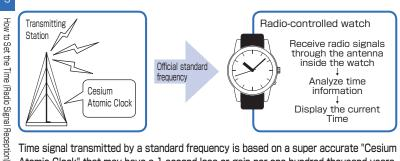
Time signal transmitted by a standard frequency is based on a super accurate "Cesium" Atomic Clock" that may have a 1 second loss or gain per one hundred thousand years.
