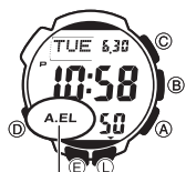
Auto light switch on indicator
