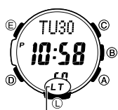
Auto light switch on indicator
