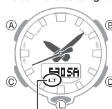
Auto light switch on indicator
